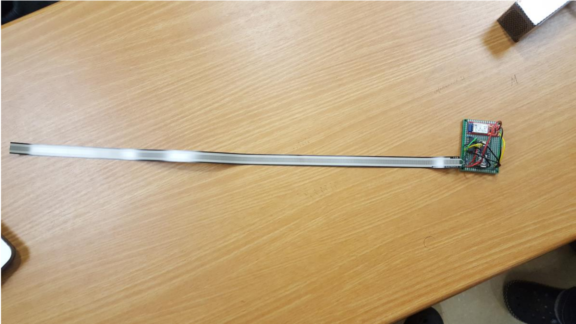
Figure 20, Connected PCB with FSR
